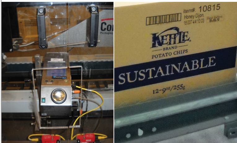
▶ (Left): A Videojet 2330 large-character printer places key data on a Kettle Foods case as it is being sealed. (Right): Printed data includes bar-code and human-readable information that includes batch code, product name, etc.
