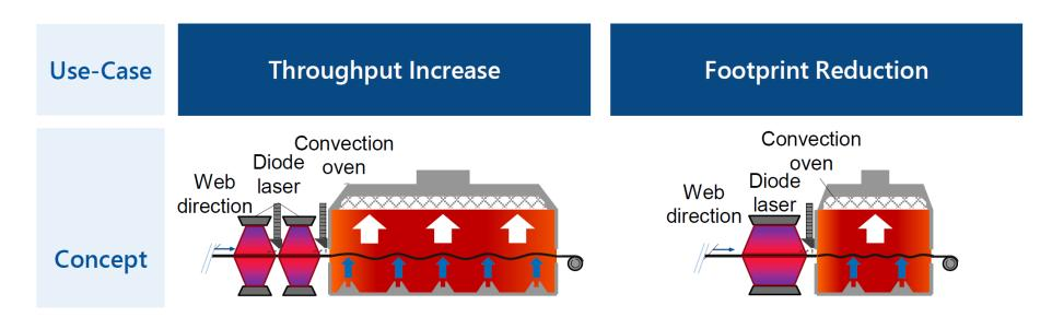
**Retrofit** – Laser pre-dried/heated product travels faster through existing long oven
