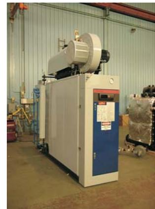
Miura's LX model has published results that show a value of 85.7% efficiency. The compact boilers' forced flow, vertical-tube pressure vessel design is more efficient, requires less heating surface, achieves higher efficiency and is less than half the size of firetube and other conventional boilers.
